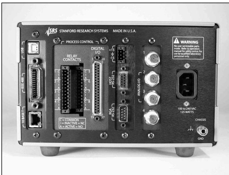
Figure 9. PPM100 Back panel. Computer interface ports on the back panel of the PPM100 include: (1) HOST RS232, (2) GPIB, (3) USB, and (4) optional Ethernet port (for embedded Webserver)
